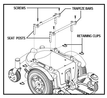
Figure 13. Seat Adjustment - Trapeze Bars
